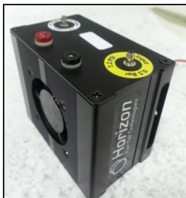
Figure 1. PEMFC Horizon H-20 with DLFC operation
