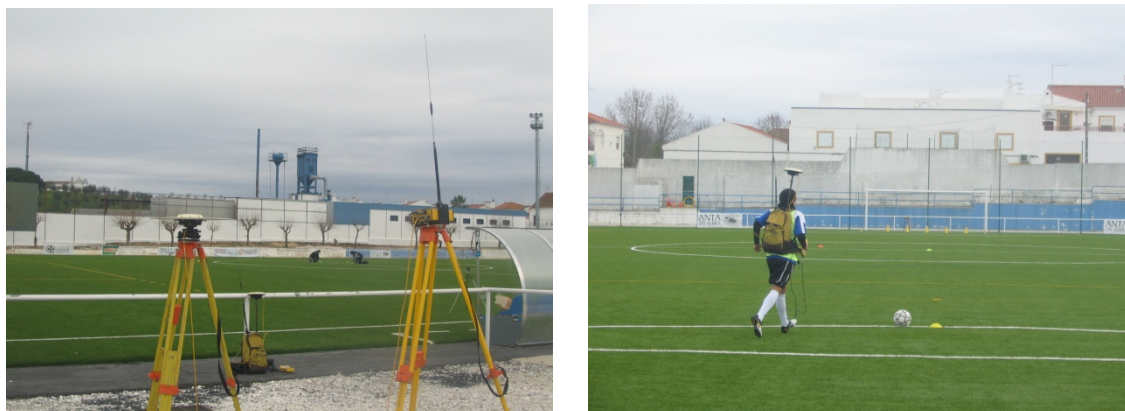
Figure 3. Differential correction station (dGPS) (top) and the football player equipped with mobile GPS antenna (bottom)
