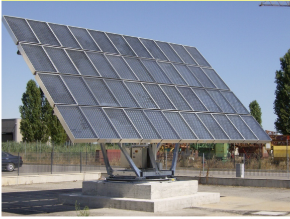
Figure 4. First installation of a 4kWp tracking Rondine Gen1 system, at Ostellato (Ferrara, Italy)
