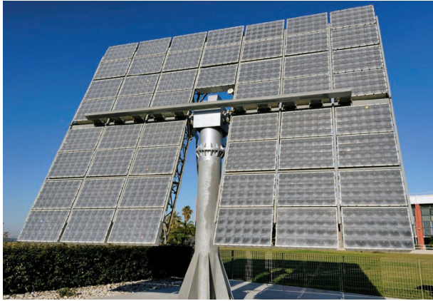
Figure 1. Standard solar PhoCUS CPV system (5 kW nominal power) installed at ENEA-Portici Laboratories (Portici, NA, Italy)
