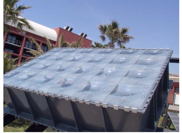
Figure 8. Photo of the PhoCUS C-Module, realized by a joint venture ENEA – EniTecnologie
