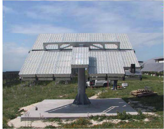
Figure 3. The new PhoCUS CPV system realized with the low-cost solar tracker, installed at ENEA-Manfredonia Laboratories
