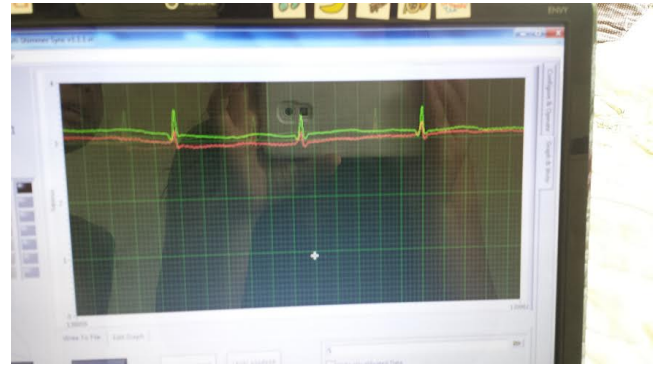
Figure 2. ECG signals on Shimmer® wireless body sensor system
