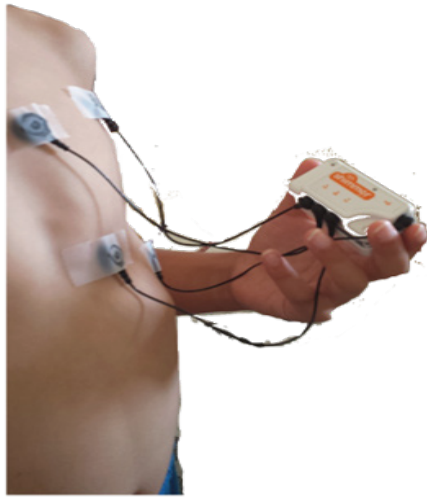
Figure 1. Shimmer® system detecting ECG signal
