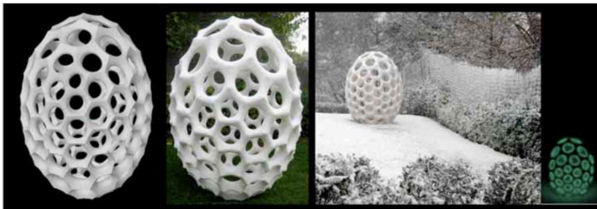
Figure 13. Biodigital Barcelona Pavilion, Barcelona, 2008-09. After “biolearning” process, CAD-CAM technologies for producing directly real 1:1 scale architecture. LEFT: Digital drawing. CENTRE / RIGHT: real CNC digitally fabricated and real installed in big architectural scale. (Right, with Biolamps application) (© Alberto T. Estévez)
