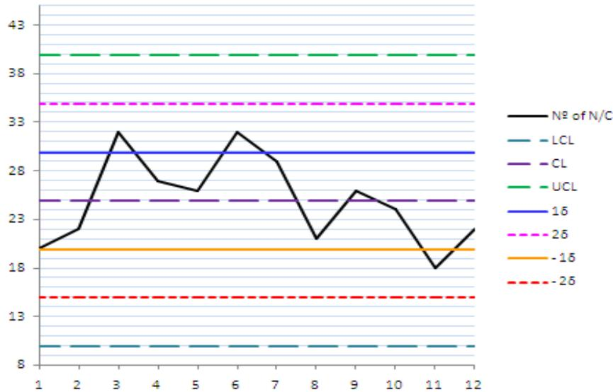
Chart 3. Type  $c$ , with the Limit and Warning Control, compared to CL
