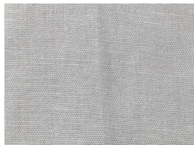
Figure 2. Plain woven (1/1 plain weave structure) cotton-flax blended RFD fabric
