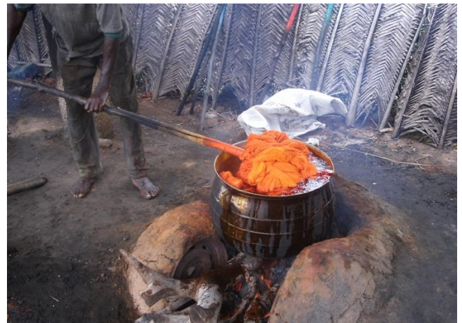
Figure 3. Yarn (hank) dyeing with reactive dye (Source: (Field Research, 2021))
