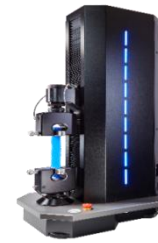
Figure 1. Universal Tensile Strength Testing Machine (James Heal)
