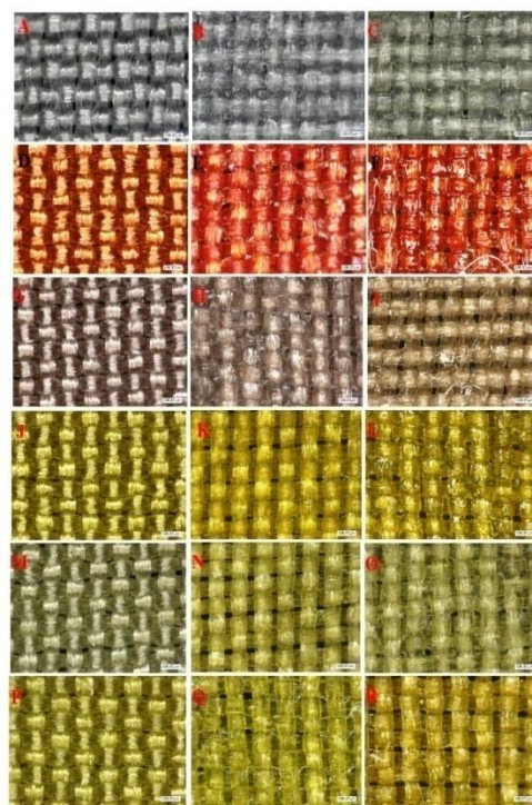
Figure 2. PVAc (Jade 403N): Microphotograph of silk fabric samples before and after UV irradiation at a magnification of \times 200 . Left control without PVAc, centre with PVAc before UV aging, and right after aging. (A, B, C) undyed, (D, E, F) dyed with Japanese madder, (G, H, I) dyed with Shikon dye, (J, K, L) dyed with Kariyasu dye, (M, N, O) dyed with Enjyu dye, (P, Q, R) dyed with Kihada dye
