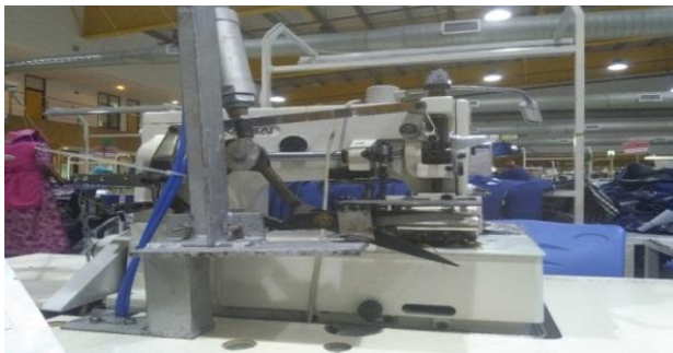
Figure 3. Adding auto thread Cutter on a Kansai machine
