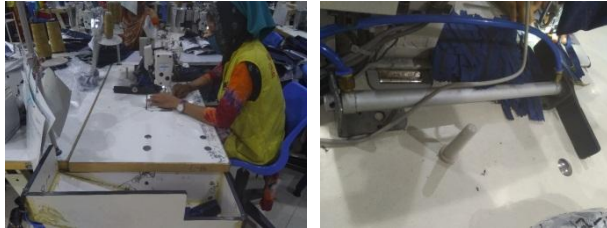
Figure 2. Added automation on double needle lock stitch machine
