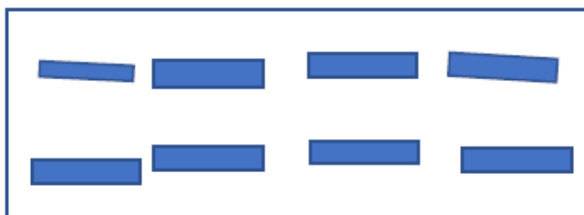
Figure 2. Parallel orientation of pigment after drying and condensation
