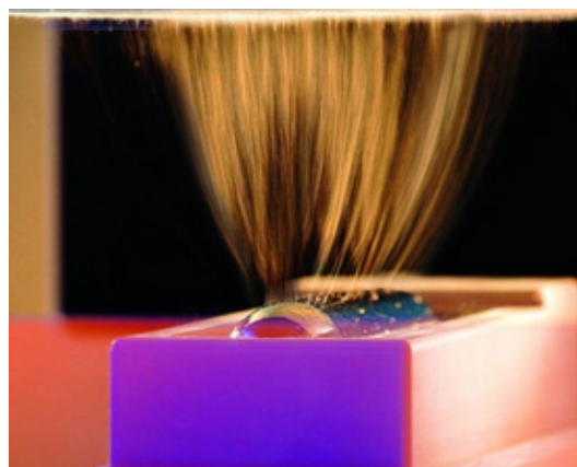
Figure 15. Rotating Roller electrospinning [34]
