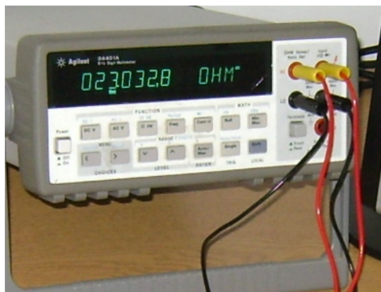
Figure 3. An Agilent Bench-top multimeter along with 4 wire resistance measurement setup
