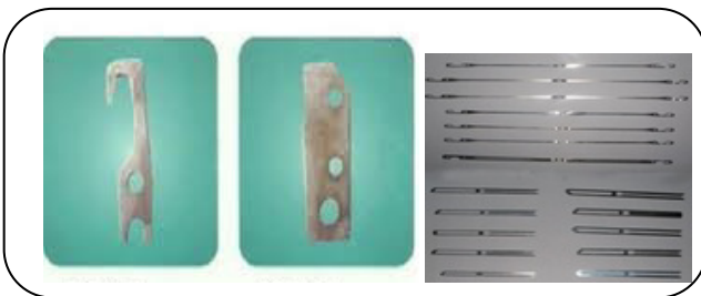
Figure 8. Different types of Drop Wire
