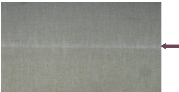
Figure 3. loom bar or starting mark (thick or dense mark)
