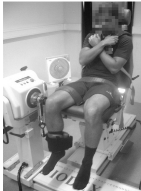
Figure 1. Positioning in isokinetic dynamometer Biodex System 4 Pro®
