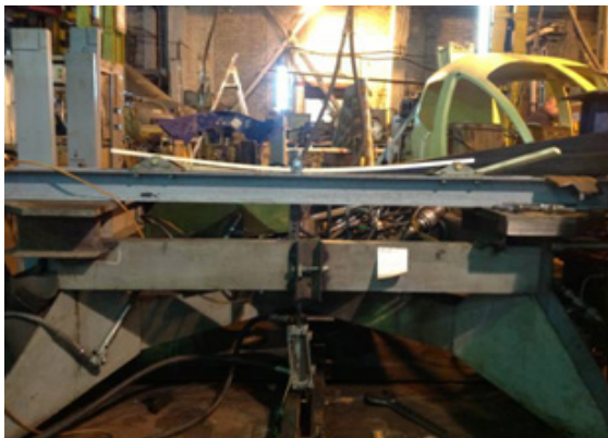
Figure 2. Testing stand imitating the ski work
