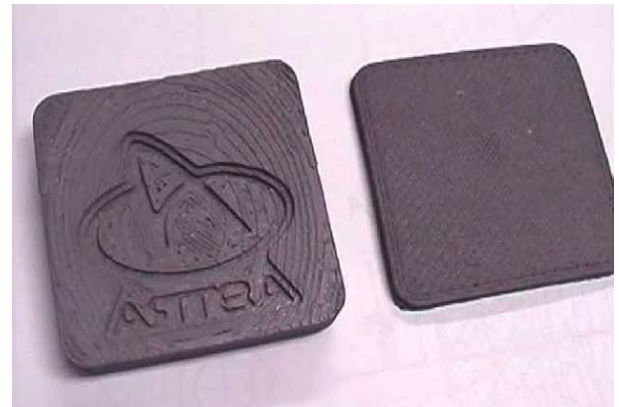
Figure 7. A complex shaped injection moulding insert produced on FDM [13]
