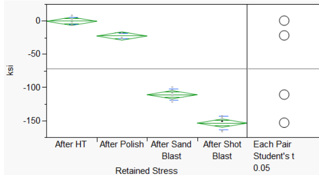
Figure 7. Residual Surface Stresses on Bearing Rings
