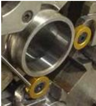
Figure 1. Supporting Ring on Outer Diameter when Grinding Inner Diameter
