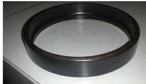
Figure 2. Scale on Tempered Bearing Ring
