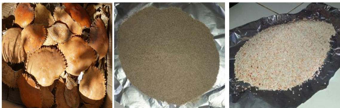
Figure 11. (A) Scylla serrata shells, (B) Ground material sieved through a 1000 µm sieve, (C) [15] [16] [17]
