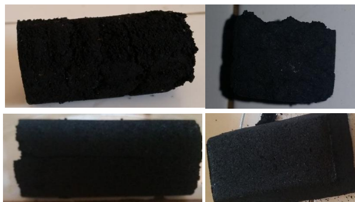
Figure 14. (A): Bio-based composite based on starch; (B) Bio-based composite based on chitosan, (C): Bio-based composite based on alginate, (D): Bio-based composite based on Cassia gum (Hervéa, 2019)
