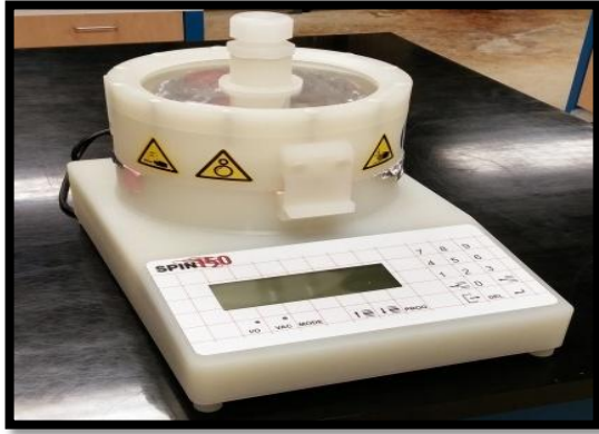
Figure 3. Front view of SPS Spin 150 spin coater
