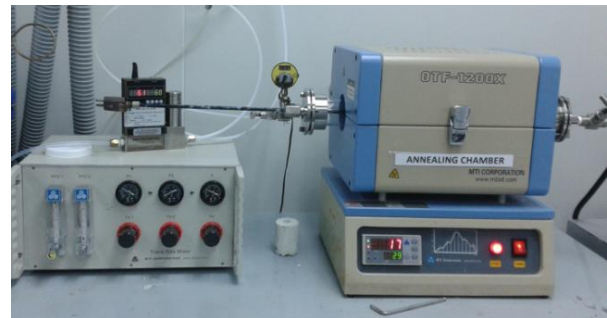
Figure 7. Diffusion Process inside the annealing chamber
