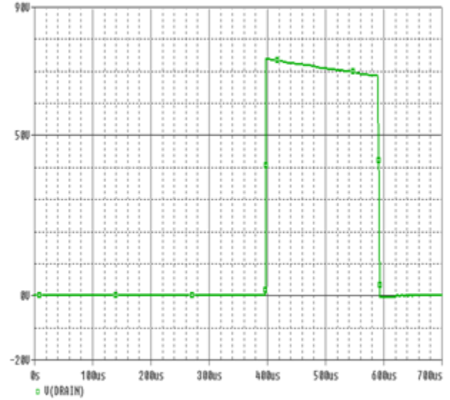
Figure 8b. Simulated drain voltage ( V_{\text{DS}} ) for the VDMOSFET transistor
