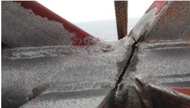
Figure (1). Crack caused by fatigue in a joint
