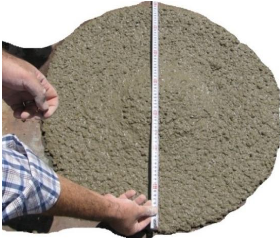
Figure 10. Slump measurement of LCHWC
