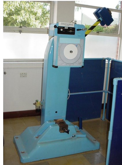
Figure 9. Gouging Abrasion Test [10]
