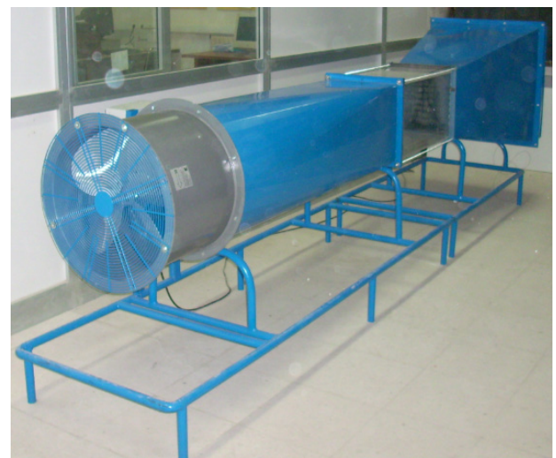
Figure 1. Experimental device of the wind tunnel
