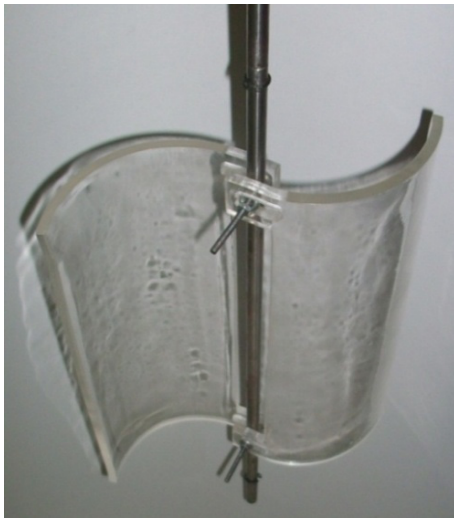
Figure 2. Incurved Savonius wind rotor
