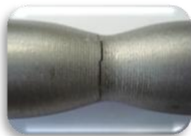
Figure 7a. Phenomena tensile steel AISI / SAE 3115: necking
