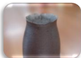
Figure 7b. Phenomena tensile steel AISI / SAE 3115: final rupture
