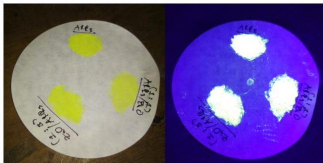
Figure 4. White Light (Left) and UV-Light (Right) exposure of \text{Alq}_3 and \text{Alq}_3/\text{ZnO} composites
