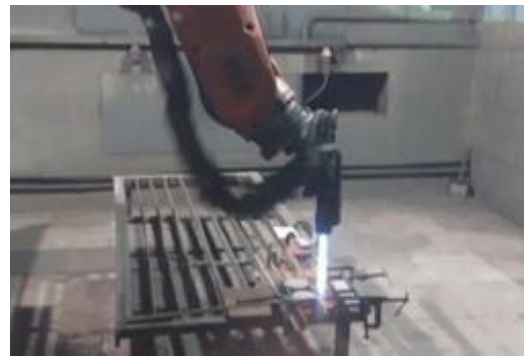
Figure 1. Application of the coating on the specimens
