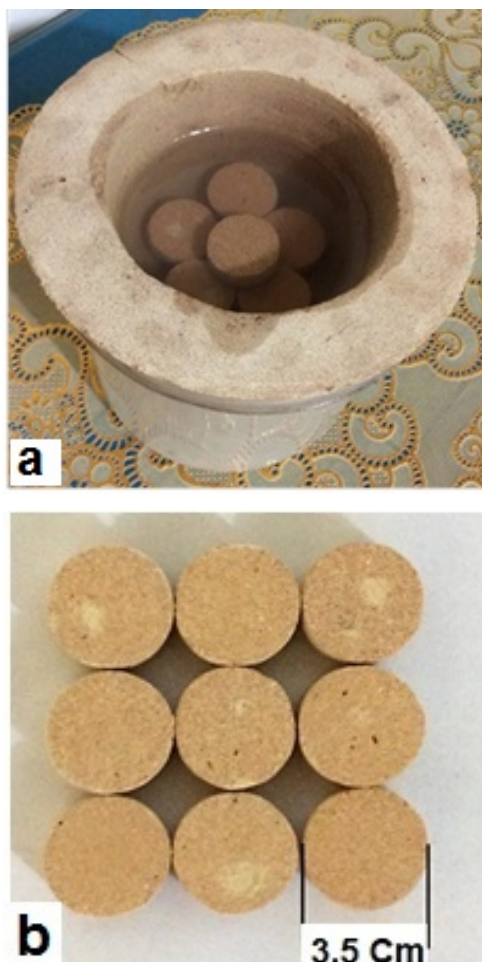
Figure 9. Filtration system, (a) Ceramic Filter with ceramic Tablets; Ceramic tablets
