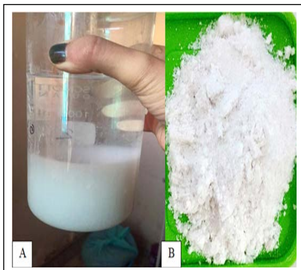
Figure 2. (a) Nanosilica before drying; (b) Nanosilica after drying for 48 hours at 50
