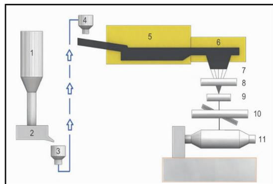
**Figure 1.** Steps involved in manufacturing of basalt fiber: 1) crushed stone silo; 2) Loading station; 3) transport system; 4) batch charging station; 5) initial melt zone; 6) secondary heat zone with precise temperature control; 7) filament forming bushings; 8) sizing applicator; 9) strand formation station; 10) fiber tensioning station; 11) automated winding station. [2, 7]
