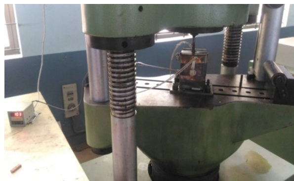
Figure 1. ECAP carried out in a UTM with heating unit
