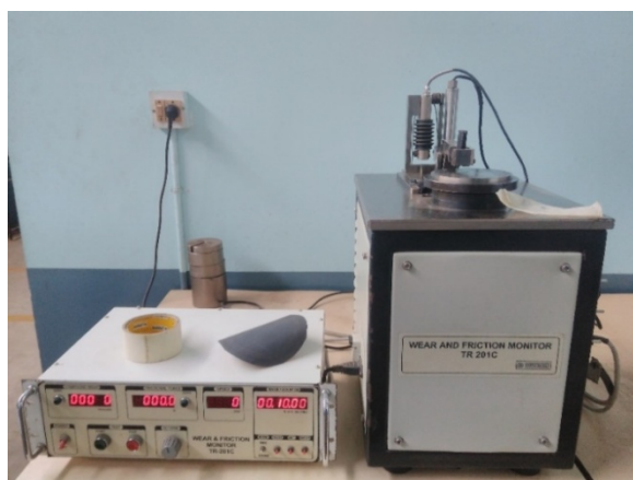
Figure 1. Wear Testing (Pin-on-Disc) setup
