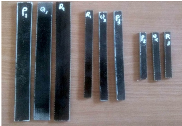
Figure 2. Hybrid composite specimen P, Q and R for Tensile, Flexural and impact test
