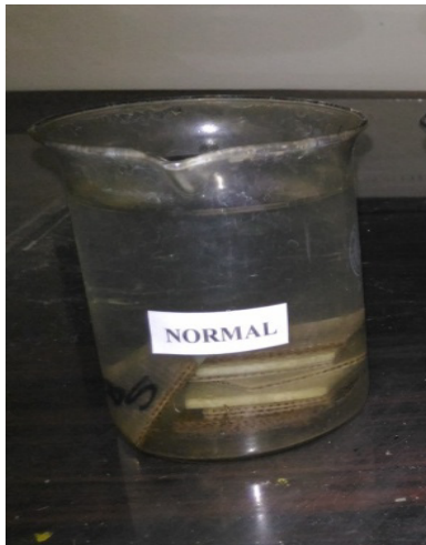
Figure 2. Test specimens immersed in normal water
