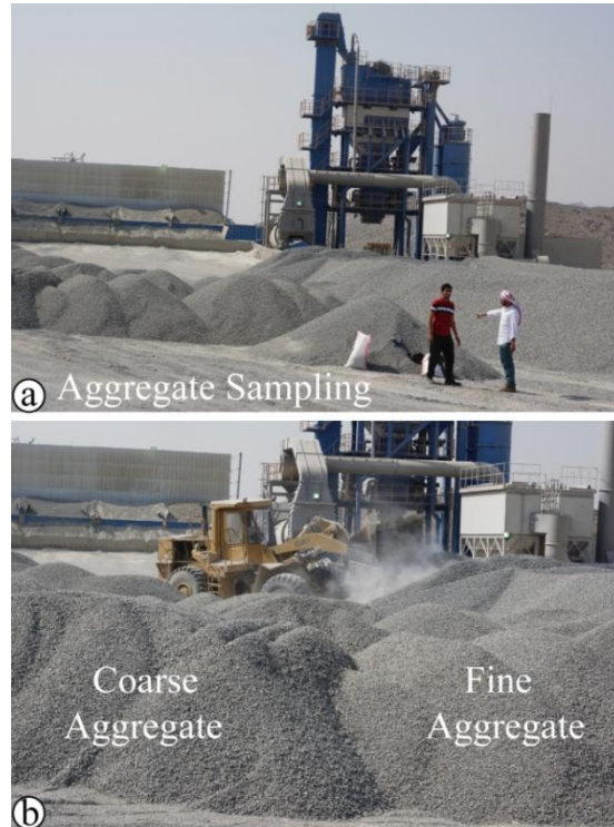
Figure 2. Field photographs show aggregate sampling and types of diorite aggregates (a and b respectively)
