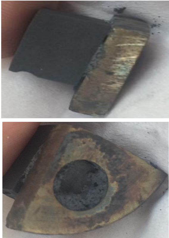
Figure 9. Interlocking braze design graphite into stainless steel
