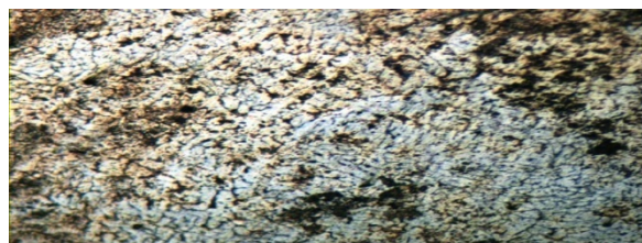
Figure 11. Microstructure of Al-2.28% Si
