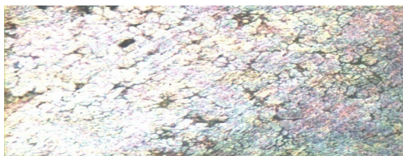
Figure 10. Microstructure of Al-0.94% Si
