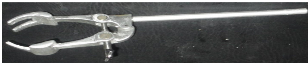
Figure 5. Fabricated three-prong extension clamp
