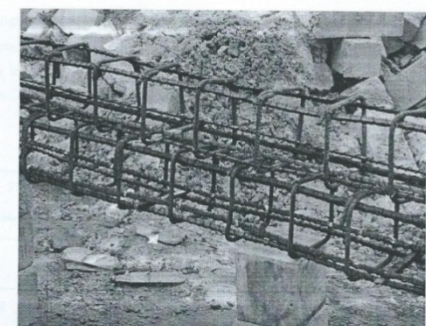
Figure 2. The arrangement of bamboo in the foamed aerated concrete beam
