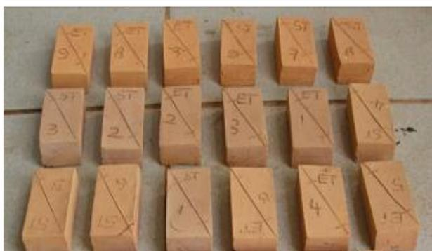
Figure 3. Bauxite Red Mud-Clay briquettes
