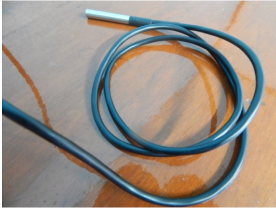
Figure 5. The DS18B20 temperature sensor used in the RWTMS
