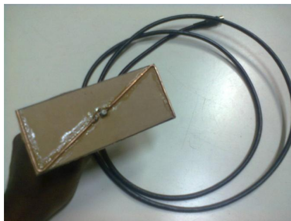
Figure 1(a). Fabricated TVWS Z Antenna in Physics Lab, Chancellor College, Malawi
