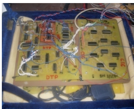
Figure 6. Interconnections of the circuit boards
