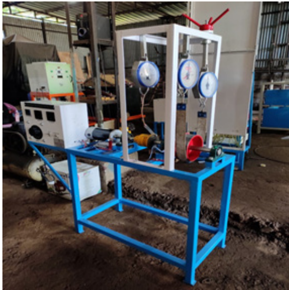
Figure 7. Epicyclic Gear Train and Torque Apparatus
