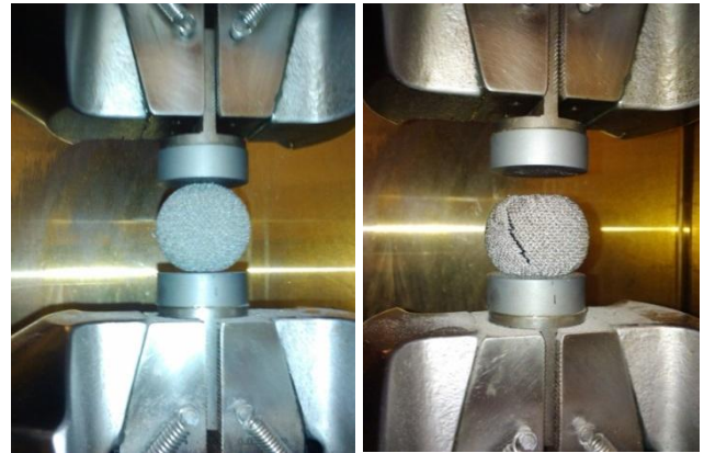
Figure 7. Load-test of one-piece titanium mesh spheres
