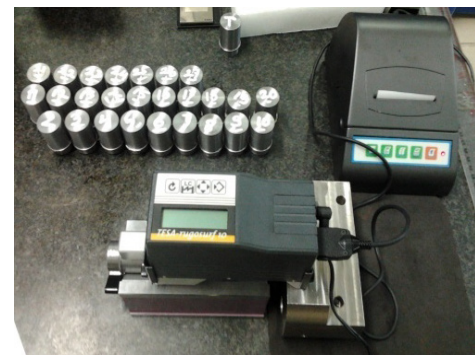
Figure 3. Surface roughness test device, Tesa Rugosurf 10 Roughness Gauge
