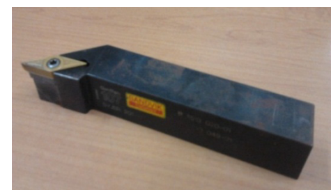
Figure 4. Cutting knife VBMT 16 - SVJBR 2020K
