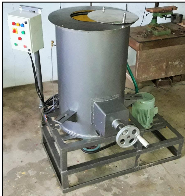
Figure 3. Photograph of the final assembled Commingled Waste Plastic Washing and Shredding Machine
