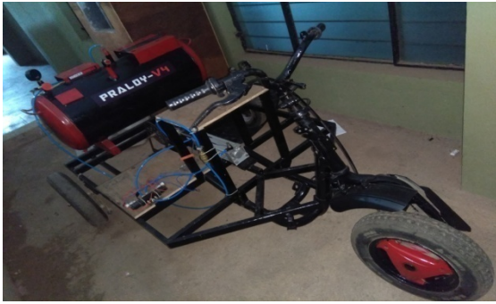
Figure 3. Prototype of air driven vehicle
